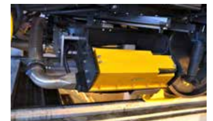
On permanent installations a fan system keeps the lenses clean
