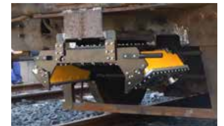
Temporary OTG installation for validation of newly laid track
