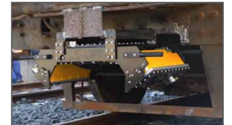
Temporary LTM installation for validation of newly laid track
